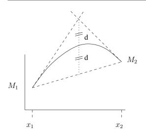
Consider a parabola passing through the points  $(x_1, M_1)$  and  $(x_2, M_2)$ . The parabola represents a bending moment diagram as a result of a constant distributed load q. The bending moment formula as a function of x is given by
