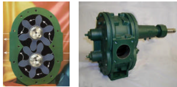
Fig. 3.8 - Displacement pump open (left) and closed (right)
