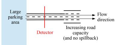
The above figure shows a simplified representation of the road layout. There is a detector at the red line, in the two-lane road stretch. Downstream of the detector the road widens and there are no further downstream bottlenecks.
