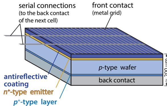
**Figure 12.8:** Scheme of a modern crystalline silicon cell.
