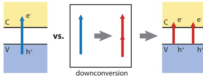
**Figure 16.2:** Illustrating the principle of spectral down-conversion.
