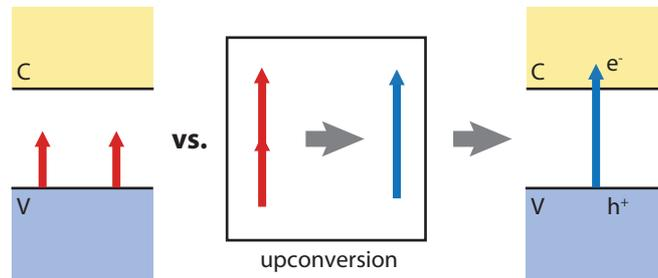
**Figure 16.1:** Illustrating the principle of spectral up-conversion.
