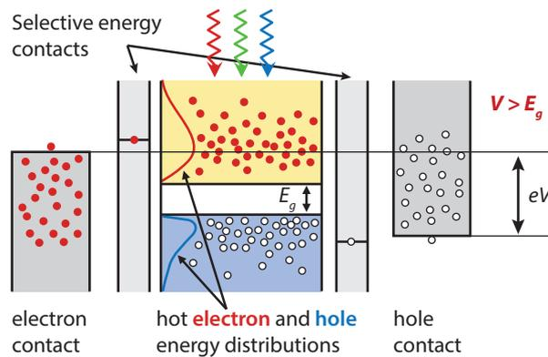
**Figure 16.8:** Illustrating the working principle of a hot carrier solar cell.
