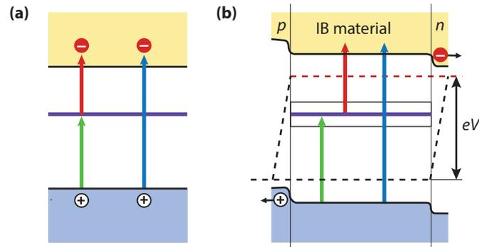
**Figure 16.7:** Band diagram (a) with the intermediate band depicted and (b) with the quasi-Fermi levels exceeding the energy of the low-energy photons.
