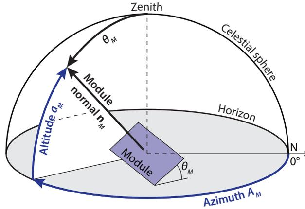
**Figure 18.6:** Illustrating the angles used to describe the orientation of a PV module installed on a horizontal plane.
