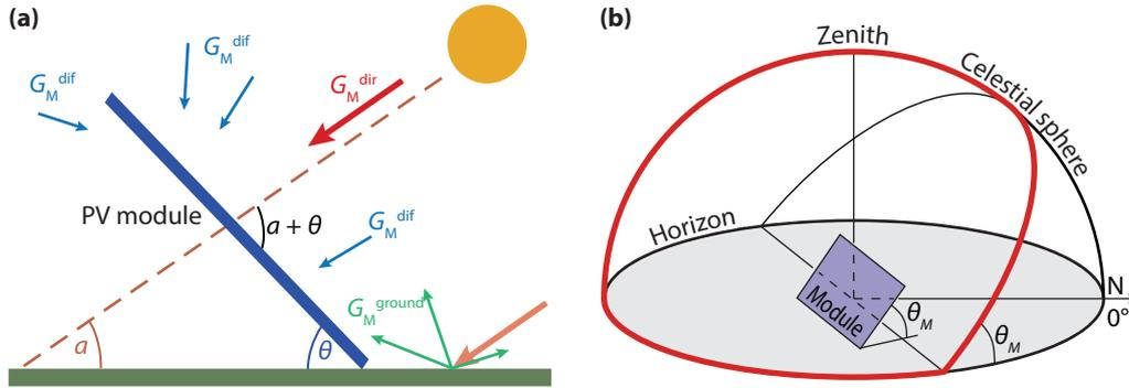
**Figure 18.7:** (a) The three contributions to the irradiance on a PV module  $G_M$ . (b) Illustrating the definition of the *sky view factor* (SVF), which is the fraction of the celestial hemisphere enclosed by the thick red line.
