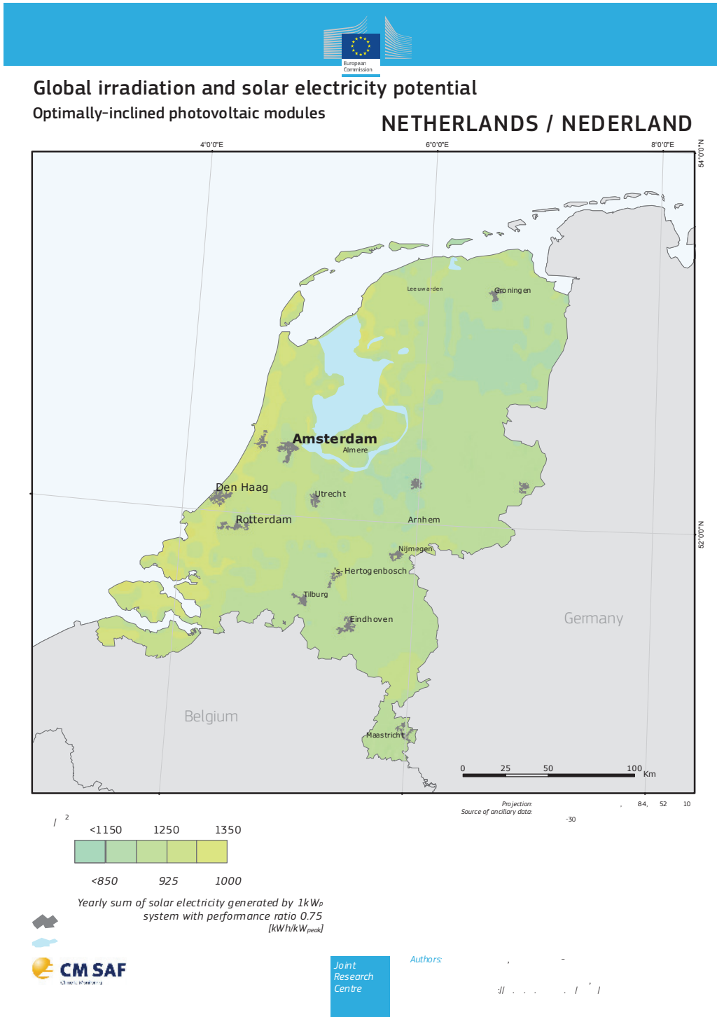
Figure 20.3: Yearly insolation at optimal tilt (36°) in the Netherlands in kWh/m 2 (Source: PVGIS [158–160]).
