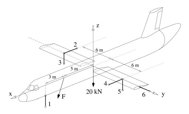
a) Calculate the forces in the six two-force members with the correct sign for tension and compression.
