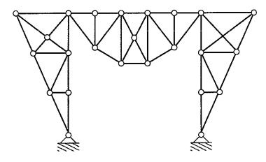
For this truss, 5>2k-3. But, remember that this is a necessary, but not a sufficient condition. In this case, the bars are placed in the wrong position.
