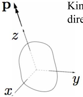
Kinematics of spinning body when direction of spin axis changes
