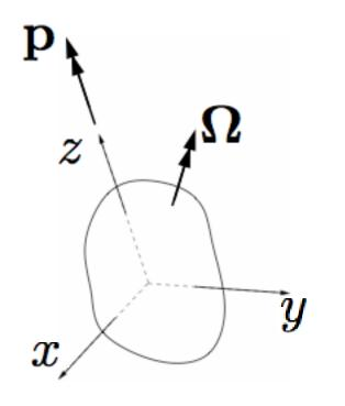
$egin{aligned} &\omega_1 &= \Omega_1 \ &\omega_2 &= \Omega_2 \ &\omega_3 &= \Omega_3 + p \end{aligned}$
