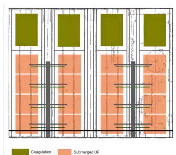
Figure 3.8: one ultra filtration street
